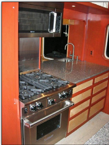
Galley upgrade with Wolf range during refit (drawer fronts not installed)
